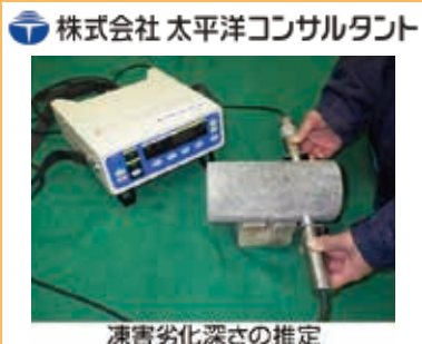
凍害劣化深さの推定
